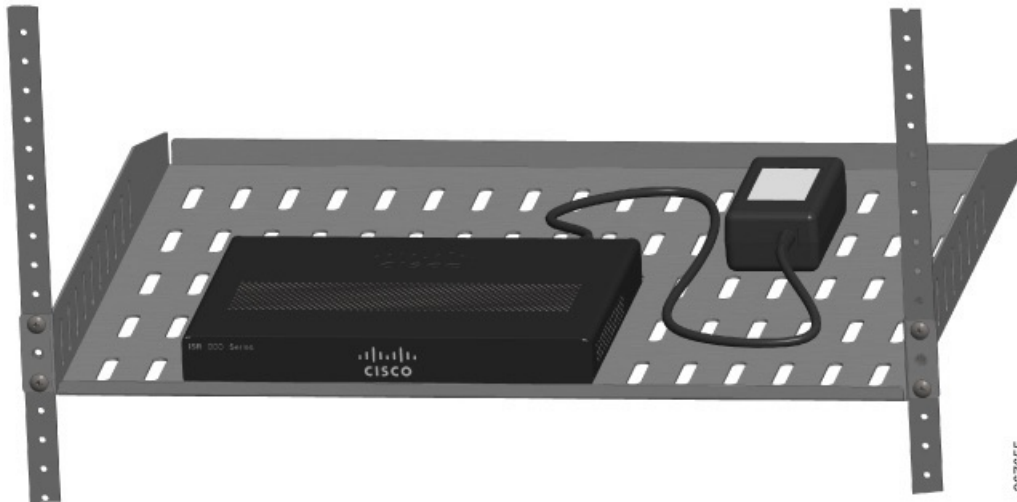
Figure 23: Mounting the Cisco ISR 900 Series Router in a Tray
